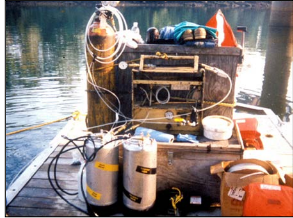
Figure 7-5 Epoxy Injection Equipment on Float
